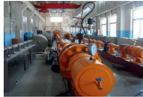
FIGURE 6: Launch platform of the 152 mm compressed-gas gun.
