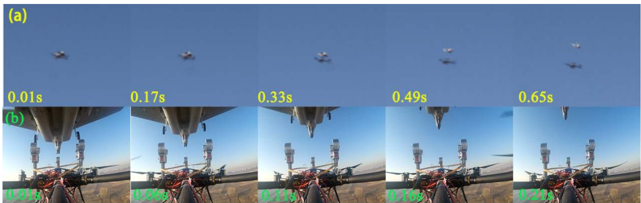
FIGURE 32. Actual separation process shot by (a) ground video equipment and by (b) airborne video equipment.
