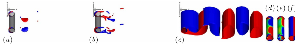
Figure 18. At t = T_1 , isosurfaces of (a) \omega_x = \pm 0.02 , (b) \omega_y = \pm 0.01 and (c) \omega_z = \pm 0.2 , and contours of (d) \omega_x , (e) \omega_y and (f) \omega_z on cylinder surfaces at Re = 160 with L_Z = 4 (same descriptions as in figure 9).
