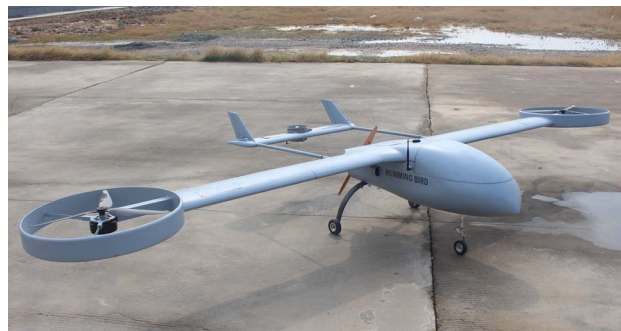
Figure 1. The tail rotor tilting three ducted fan VTOL-UAV.
