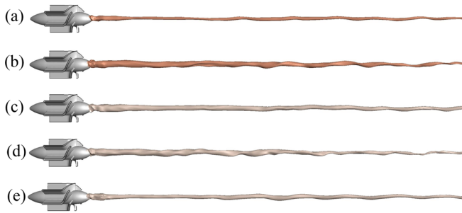
FIG. 9. Gas column distribution under different fluid rheology parameters [(a) k = 0.01337 \text{ Pa s}^n , n = 0.08056 , \alpha_{giso} = 0.8 , Re = 25447 ; (b) k = 0.01337 \text{ Pa s}^n , n = 0.80557 , \alpha_{giso} = 0.8 , Re = 6997 ; (c) n = 0.02 \text{ Pa s}^n , n = 0.65 , \alpha_{giso} = 0.65 , Re = 5836 ; (d) k = 0.02 \text{ Pa s}^n , n = 0.89 , \alpha_{giso} = 0.65 , Re = 3732 ; and (e) pure water, \alpha_{giso} = 0.65 , Re = 64280 ].
