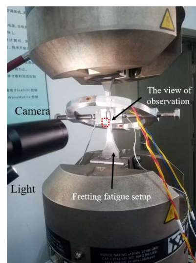
Figure 3. Photograph of the complete experimental setup in this study (The magnified area of the red wireframe is the field of view observed by the camera).
