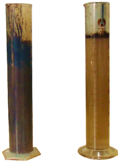
Fig. 18. One of the sampling results at overflow port and underflow port.
