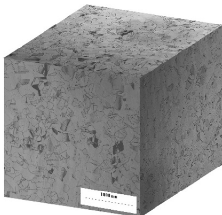
Fig. 1. Metallograph of domestic 316LN stainless steel.
