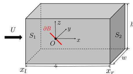
**FIG. 2.** The rectangular computational domain for the flow past a plate with six surfaces, where  $S_1$  is the upstream surface at  $x = x_l$  and  $S_2$  is the downstream surface at  $x = x_r$ , with the height  $h$  and width  $w$ . The red line denotes the plate bounded by the surface  $\partial B$ .
