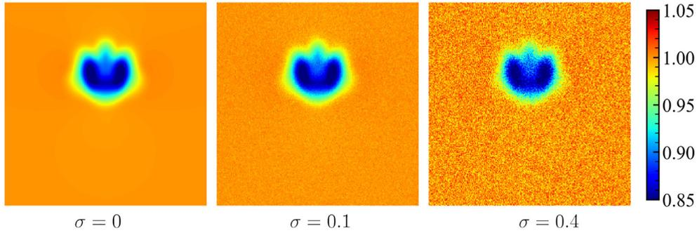
FIG. 21. Comparison of contours  $u_{s,x}$  of synthetic data with different noise levels at  $x = 10$  for the flow past a stationary plate with  $\alpha = 30^\circ$ .
