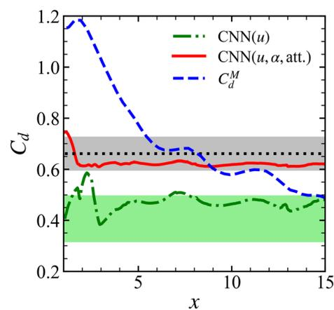
**FIG. 13.** Comparison of the CNN models in Table IV and theoretical model in Eq. (26) for estimating  $C_d$  in DNS case with  $\alpha = 40^\circ$ . The gray shade denotes 10% relative error, and the green shade denotes the range of  $C_d$  in the training set.
