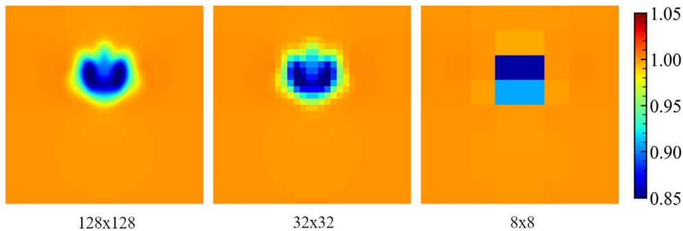
FIG. 22. The comparison of  $u_x$  with different mesh resolutions at  $x = 10$  for the DNS case with  $\alpha = 30^\circ$ .
