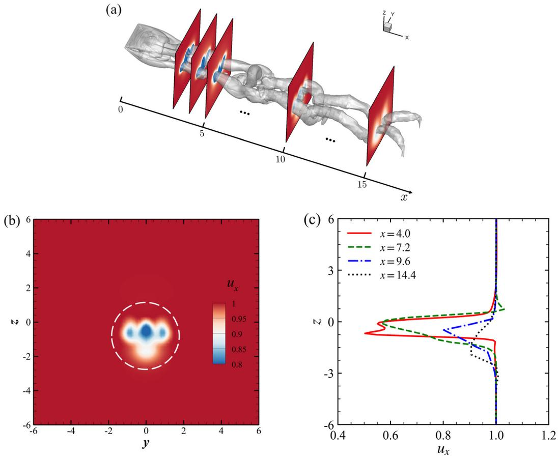
**FIG. 3.** Wake structures in the flow past a stationary plate with  $Re = 300$ ,  $R_A = 2$ , and  $\alpha = 30^\circ$  at  $t = 35$ . (a) Isosurface of  $Q = 0.02$  and contours of  $u_x$  on a series of cross sections along  $x$ . (b) Contour of  $u_x$  on the cross section at  $x = 10$ . (c) Profiles of  $u_x$  along the  $z$  direction at  $y = 0$  at different  $x$ .
