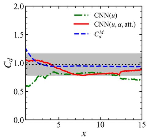
FIG. 18. Comparison of theoretical and CNN models for estimating thrust of the flapping elliptical plate at different  $x$ . The gray shade denotes 20% relative error.
