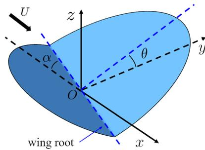
FIG. 16. Schematic of the flow past a butterfly-like elliptical plate with the angle of attack  $\alpha$  and flapping angle  $\theta$ .
