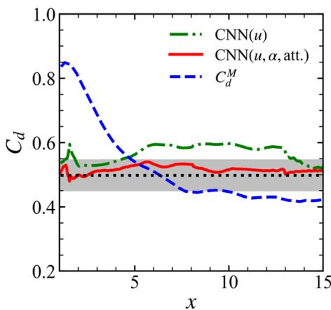
**FIG. 12.** Comparison of the CNN models in Table IV and theoretical model in Eq. (26) for estimating  $C_d$  in DNS case with  $\alpha = 30^\circ$ . The gray shade denotes 10% relative error.
