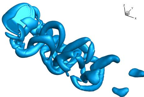
FIG. 17. Isosurface of  $Q = 1$  for the flow past a butterfly-like elliptical plate.
