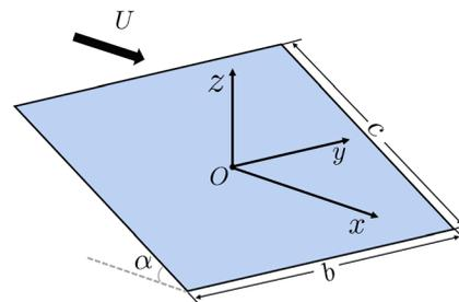
FIG. 1. Schematic of the flow past a plate with the coordinate system  $O$ - $xyz$ .
