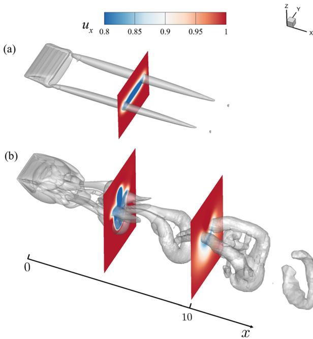
FIG. 4. Isosurfaces of  $Q=0.02$  and contours of  $u_x$  on  $y-z$  planes in the flow past a stationary plate with  $Re=300$ ,  $R_A=2$ , and (a)  $\alpha=5^\circ$  and (b)  $\alpha=40^\circ$ .
