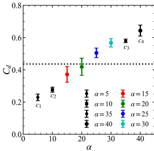
**FIG. 19.** Data of  $C_d$  in the training set (in black) and estimations of  $C_d$  from the model  $\text{CNN}(\mathbf{u})$  and the validation set (in color) of  $D_1$  for the stationary plate, where  $c_1 \sim c_4$  are labels of the four cases in the training set. The error bar denotes the standard deviation. The dotted line denotes the modeling result from the random classifier.
