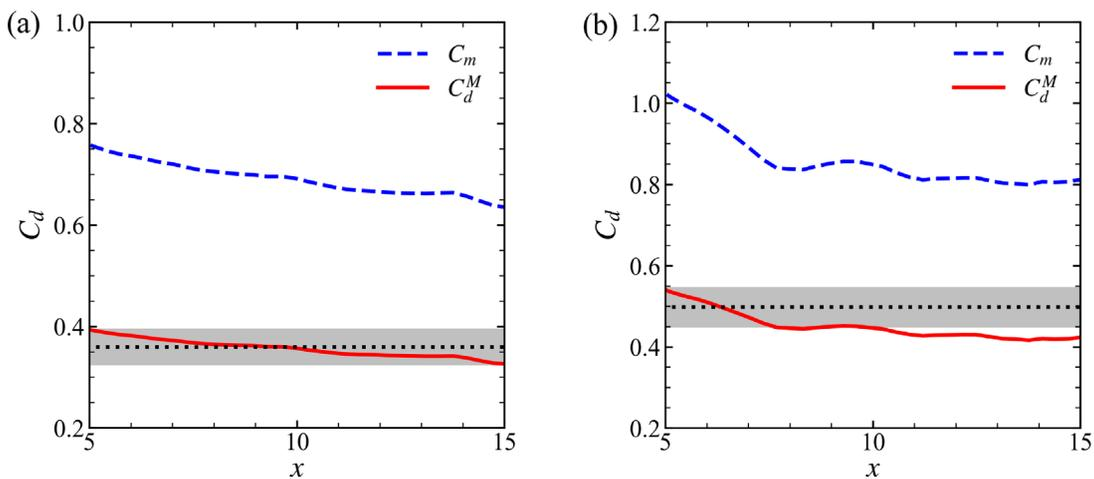
FIG. 5. Comparison of theoretical models of  $C_d^M$  in Eq. (26) and  $C_m$  in Eq. (27) based on wake cross-sectional velocity field along  $x$  with (a)  $\alpha=20^\circ$  and (b)  $\alpha=30^\circ$ . The gray shade denotes 10% relative error. The dotted line denotes  $C_d^{DNS}$ .
