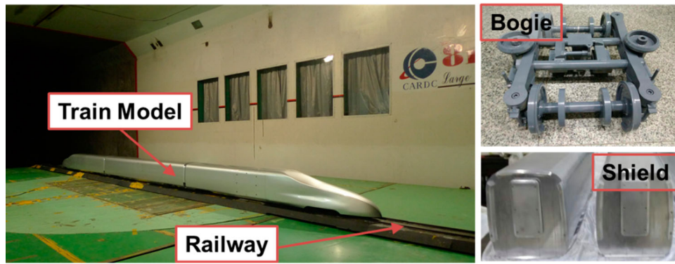
Figure 14. Wind tunnel test.
