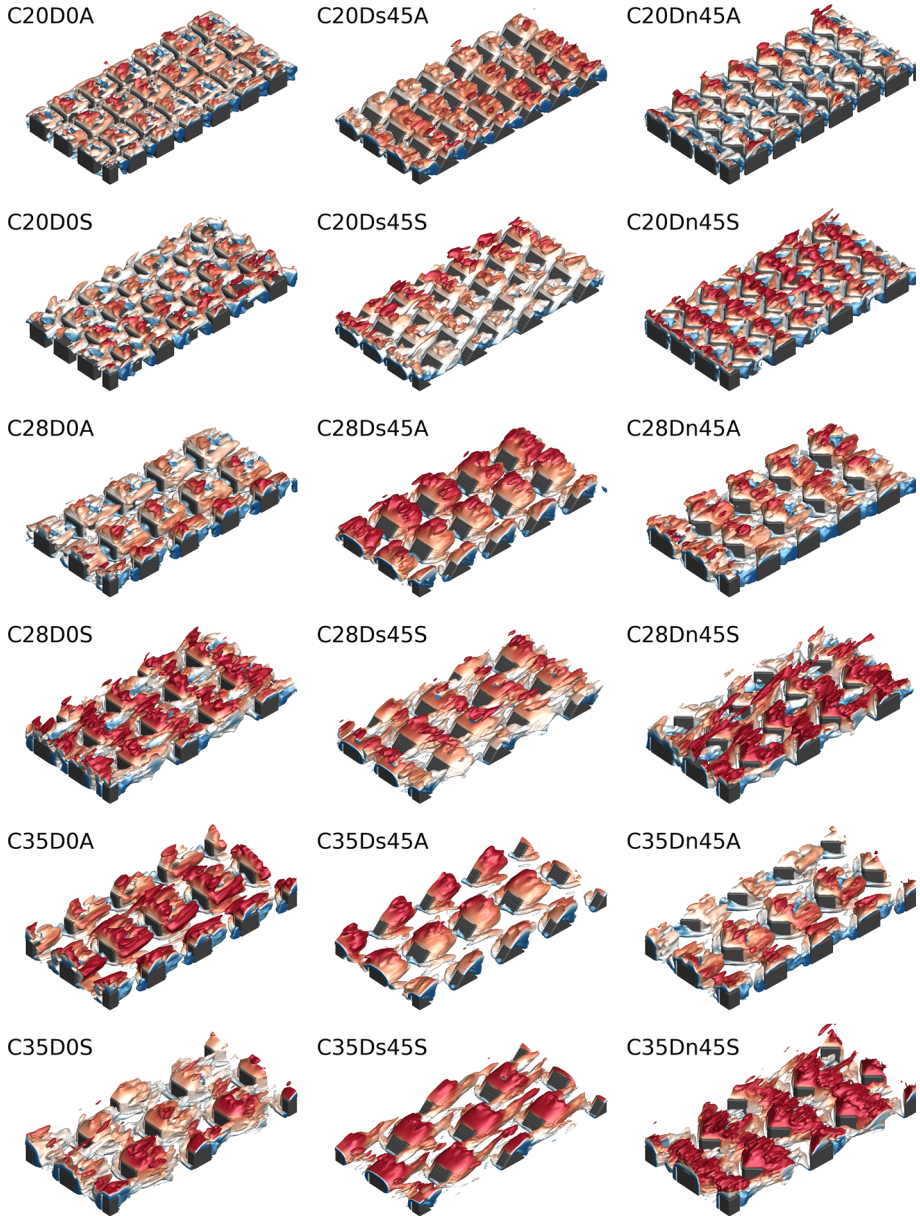
Fig. 4 Near-wall time-averaged flow structures visualized using the \lambda_2 criterion ( \lambda_2 = -0.5 ). The iso-surfaces are colored using the time-averaged streamwise velocity. Only a part of the domain is shown in the figure
