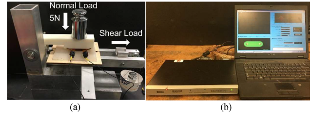
Fig. 7. (a) Real test setup with copper fingertip. (b) Signal generation and data acquisition system for the slip test setup.
