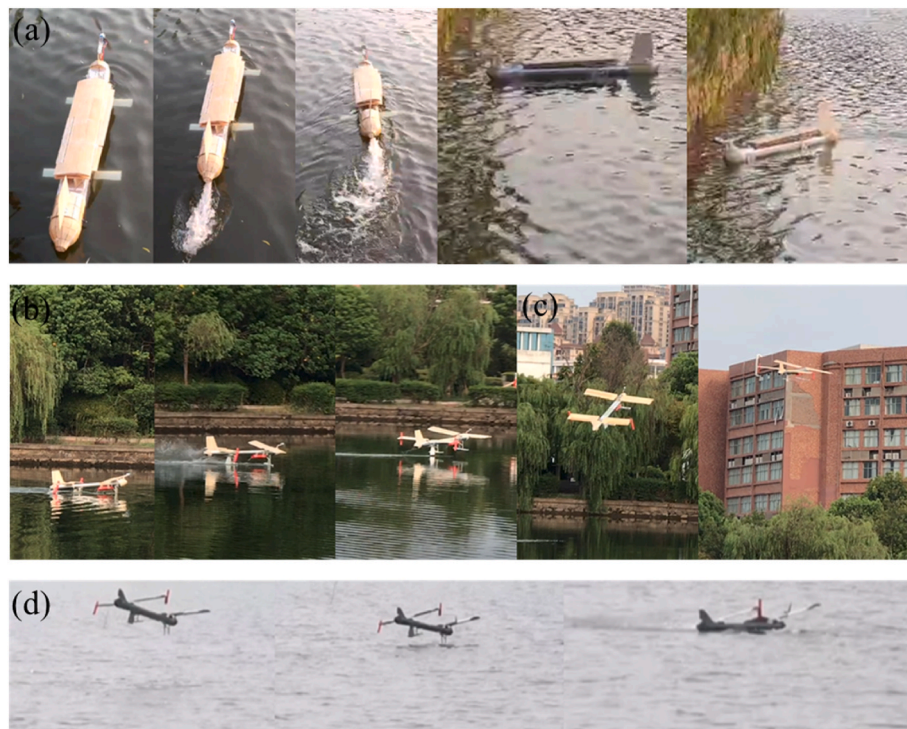
Fig. 16. The cross-domain experiment of CDV on the lake (detailed experimental process see supplementary movie). (a) Surface sailing and steering; (b) high speed sailing and take-off; (c) flying in the air; (d) landing on water surface.
