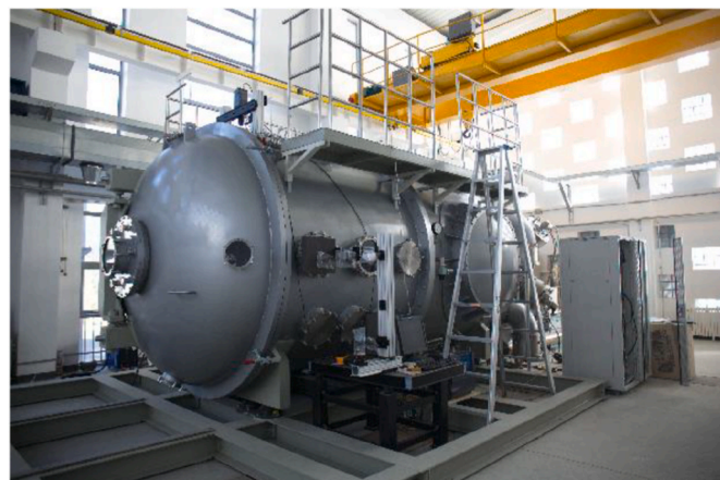
Fig. 1. Long-term ultrahigh-speed rarefied gas wind tunnel at the Institute of Mechanics, Chinese Academy of Sciences.
