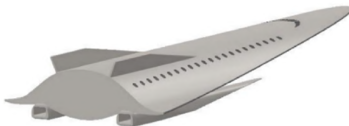
(b) Hypersonic waverider vehicle with deformable scramjet
