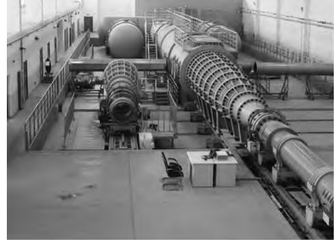
图 1 JF-12 复现风洞(图片来源:参考文献[27]) Fig.1 JF-12 shock tunnel (Source: reference [27])
