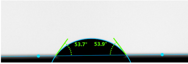
FIG. 2. Contact angle measurement results of a 3D printed flat plate.
