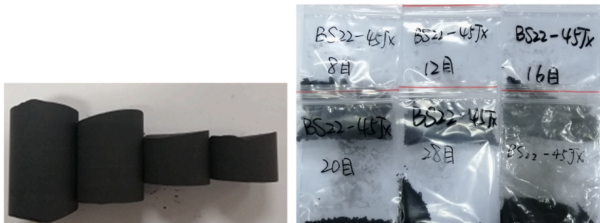
Fig. 2. The cylindrical and crushed & sieved samples with different particle sizes.
