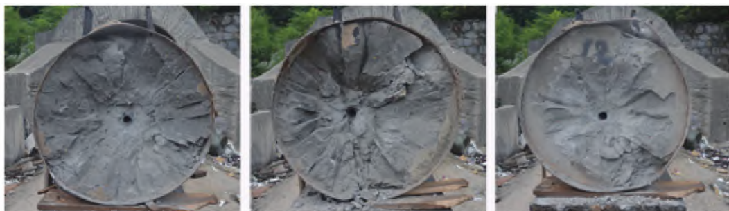
(a) Hf-based amorphous alloy-W alloy jacketed LRP ( v=1\ 415\ \text{m/s} )
