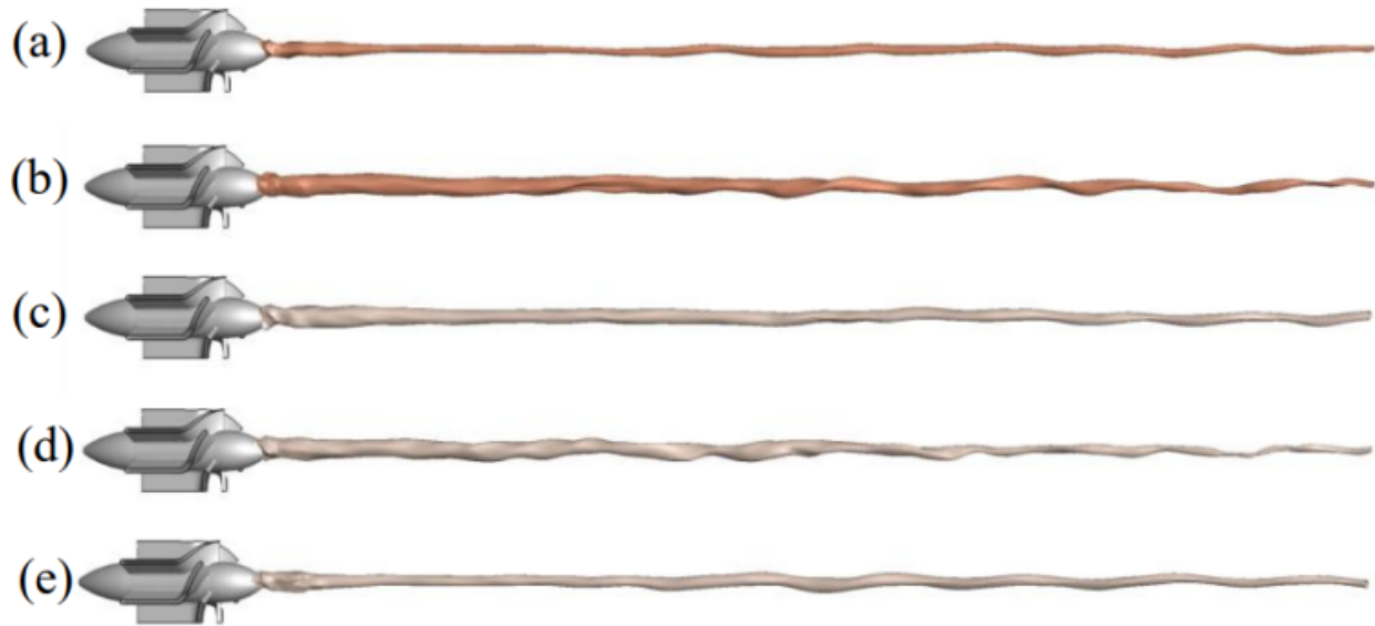
图12 不同幂率参数条件下的气液界面形状 ( a. k=0.01337 \text{ Pa}\cdot\text{s}^n , n=0.08056 , \alpha_{giso}=0.8 , Re=25447 ; b. k=0.01337 \text{ Pa}\cdot\text{s}^n , n=0.08056 , \alpha_{giso}=0.8 , Re=6997 ; c. k=0.02 \text{ Pa}\cdot\text{s}^n , n=0.65 , \alpha_{giso}=0.65 , Re=5836 ; d. k=0.02 \text{ Pa}\cdot\text{s}^n , n=0.89 , \alpha_{giso}=0.65 , Re=3732 ; e. 纯水, \alpha_{giso}=0.65 , Re=64280 ) [6]
