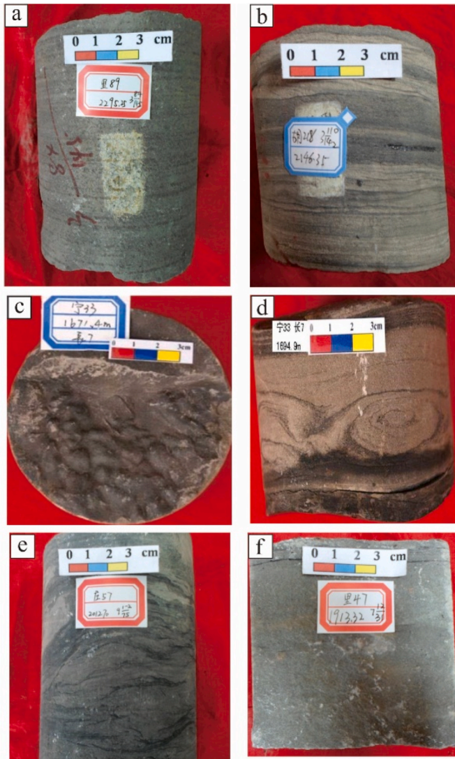
Fig. 5. Sedimentological characteristics of cores in the Chang 7 sandstones. a) Parallel bedding, L-8, 2295.25 m; b) ripple bedding, H-2, 2146.35 m; c) load structures, NG-3, 1671.4 m; d) convolute bedding, NG-3, 1694.9 m; e) slump deformation, ZH-5, 2012.7 m; f) massive sandstones, L-4, 1913.32 m.
