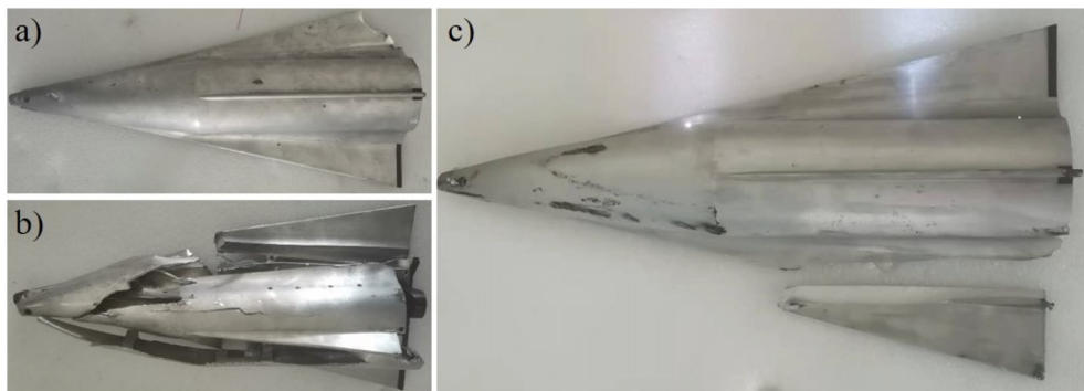
FIG. 9. The damaged orbiter models in the tests.
