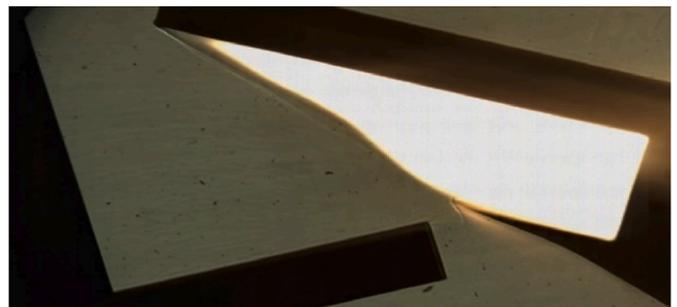
Fig. 24. Experimental photo of the oblique detonation standing in the combustor of the sodramjet engine test model for Mach number 9 [16].
