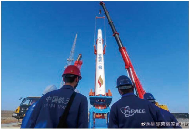
图8 “双曲线”一号遥六火箭单吊车翻转架起竖
