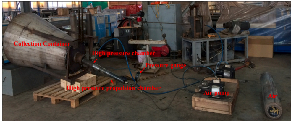
Fig. 2. Experiment apparatus for ore pulverization.
