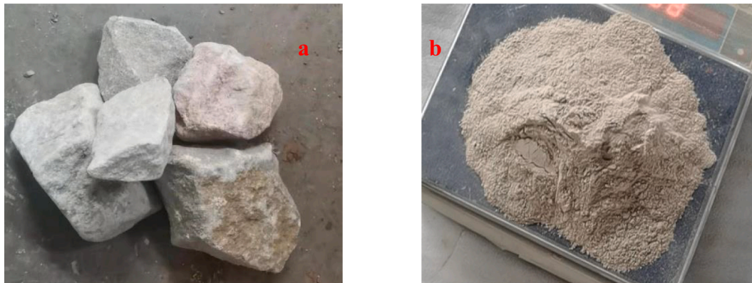
Fig. 3. Quartz sandstone before and after the experiment. (a) The quartz sandstone (b) The quartz sandstone powder.
